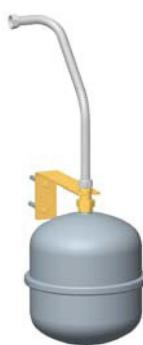
5. Connect the connecting pipeline for the expansion tank below the safety valve and fix the bracket for the expansion tank.
